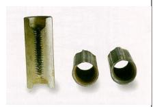
An example of coupling wear as a result of not running rod rotators
