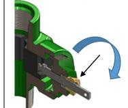
Step 6 of 6: to fully disengage repeat steps 1 -2 in order to open rams back up for operation.
