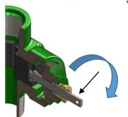
Step 4 of 5: Turn ram bolt clockwise 1-2 times. Repeat on opposite side. Continue turning 1-2 times alternating sides until rams are fully engaged.
