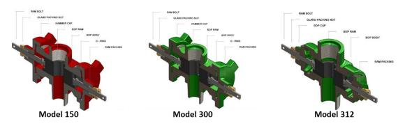
Factory settings for BOPs are male pin down. BOP rams are marked with "THIS SIDE UP" stickers. If BOP is installed female box down rams must be turned over so that "THIS SIDE IP" is facing up.
