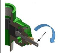
Step 5 of 5: Once rams are fully engaged tighten packing gland 1-2 turns. Repeat on opposite side. \*Continue to tighten packing gland, if necessary by ½ turns to stop leaks.
